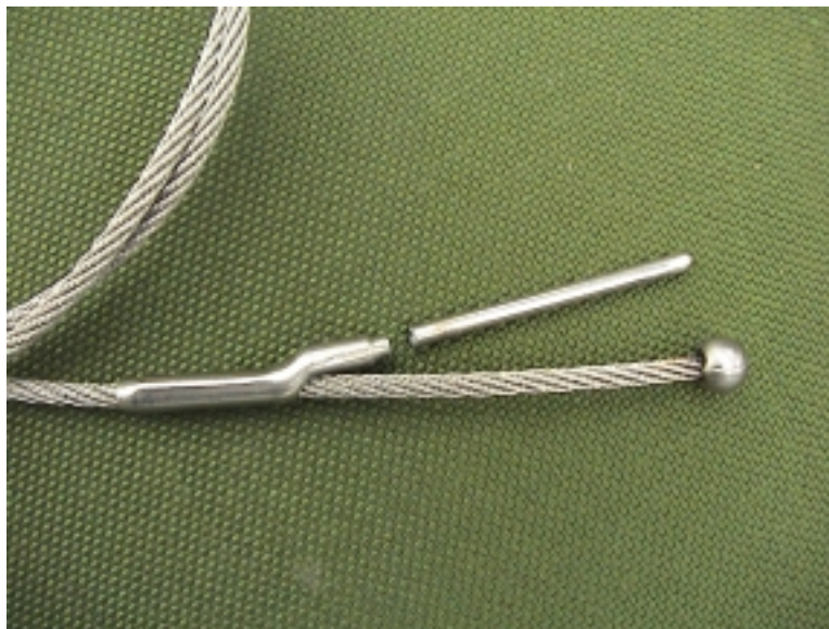
Broken Ripcord Pin
